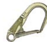
FP-RL20-C Coated Snap Hook • Exceeds ANSI Z359.1 standards. • Stainless steel gate. • 25/32" Gate opening.
